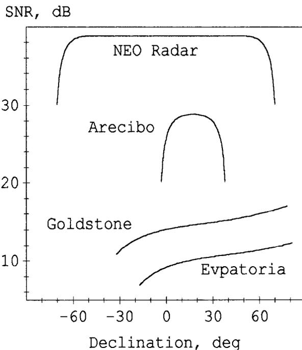
**Fig. 9.** Echo strength and sky coverage for Arecibo, Goldstone, and Evpatoria, compared to that of a proposed dedicated radar telescope. The signal-to-noise ratio is calculated for a typical kilometer-size asteroid at 0.1 AU
